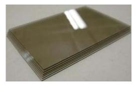
Using the Fantom G4 Laser Glass Scriber, equipped with a continuous wave 200 watt Co2 laser, rectangular glass samples were processed. Operating at 50% power, the samples were cut at a rate of 300mm per second and in one pass. After the G4 made the microcrack in the glass, the samples were then broken by hand.
